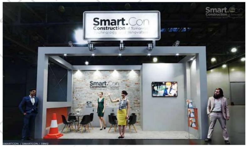
FLOOR: Gray carpet applied on local floor Walls / Semi Ceilings - Ceilings Stand built in joinery system. With rigging battens, plywood sheets and MDF, covered by nappa. Details with wire rope and screens. 1 storage with shelves and lockable door access
